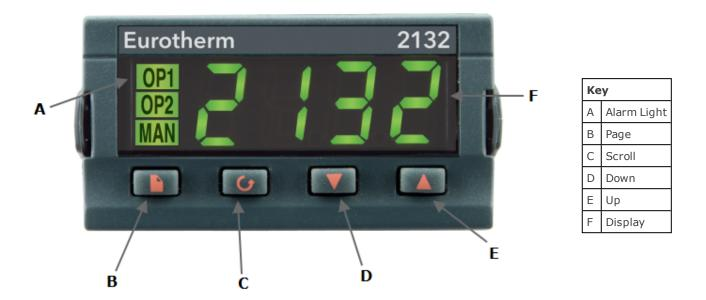
This over-temperature controller is fitted and supplied ready to use by Carbolite Gero. It is a digital instrument with a latching alarm, requiring no additional panel controls. The controller features easy setting of over-temperature setpoint and reading of current temperature by the over-temperature sensor.
